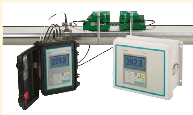
Figure 1. By measuring the difference in the speed of sound transmitted and received (transit time), these ultrasonic meters measure velocity and compute flow.
